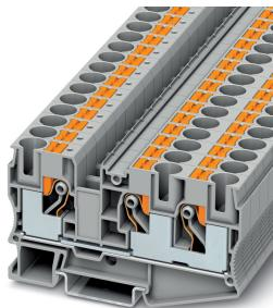
Feed-through terminal block, nom. voltage: 1000 V, nominal current: 57 A, connection method: Push-in connection, 1 level, Rated cross section: 10 mm<sup>2</sup>, cross section: 0.5 mm<sup>2</sup> - 16 mm<sup>2</sup>, mounting type: NS 35/7,5, NS 35/15, color: gray
